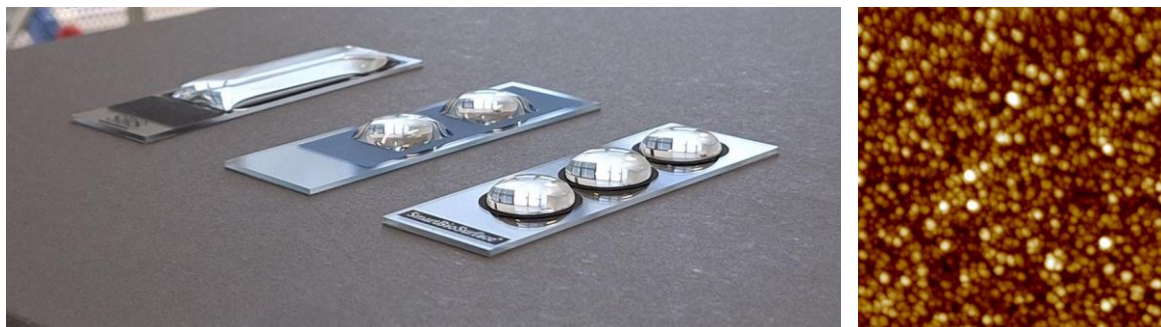
Figure 1. SmartBioSurface® slides. Left Image: SmartBioSurface® slides in a different format. Right Image: Atomic Force Microscopy (AFM) of the nanocoating (50 nm thickness)
