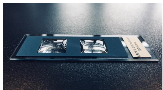
Fig. 2. Image of a SBS slide with 200 \mu\text{L} of cell solution pipetted onto each of the cell deposition areas.
