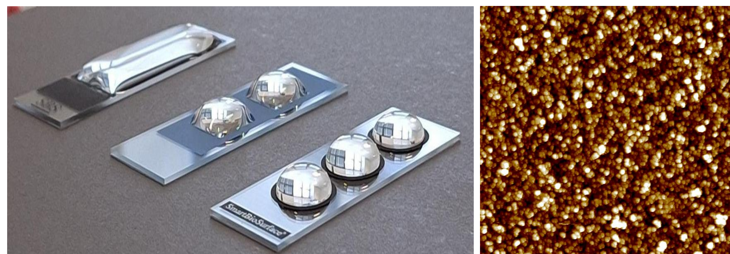
Left Image: SmartBioSurface® slides in different formats. Right Image: Atomic Force Microscopy (AFM) of the nanostructured titanium surface showing homogeneous nanoscale features.; thickness: 47.6 \pm 5.68 nm; specific surface area*: 1.38 \pm 0.03 ; RMS roughness: 9.5 \pm 0.1 nm. *Specific surface area is defined as the ratio between 3D surface area and projected scan area.
