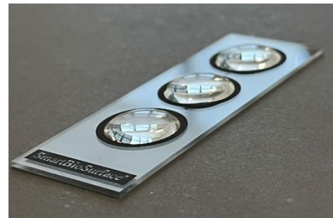
Fig. 2. Image of a SmartBioSurface® slide with 150 µL of cell solution pipetted onto each of the cell deposition
