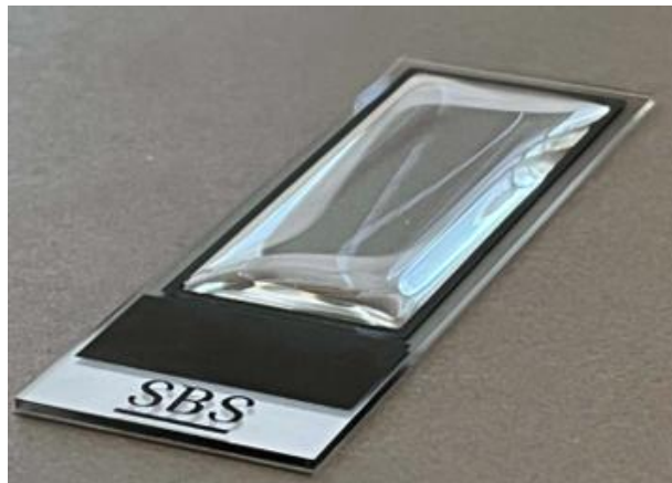
Fig. 1. Image of a SmartBioSurface slide with 800 \mu L of cell solution pipetted the cell deposition areas.
