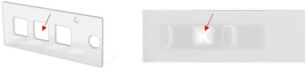
Figure2. Cell deposition on SmartBioSurface. Left: reusable CultureWell™ silicone gasket used to define the deposition area. Right: SmartBioSurface slide showing the gasket-defined deposition area (red arrow), where the enriched cell suspension was seeded, incubated for spontaneous cell adhesion and fixed with formaldehyde 4%.
