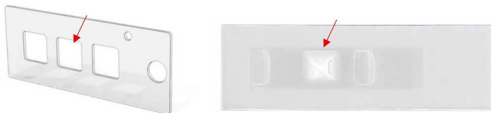
Figure2. Cell deposition on SmartBioSurface. Left: reusable CultureWell™ silicone gasket used to define the deposition area. Right: SmartBioSurface slide showing the gasket-defined deposition area (red arrow), where the enriched cell suspension was seeded, incubated for spontaneous cell adhesion and fixed with 4% PFA.
